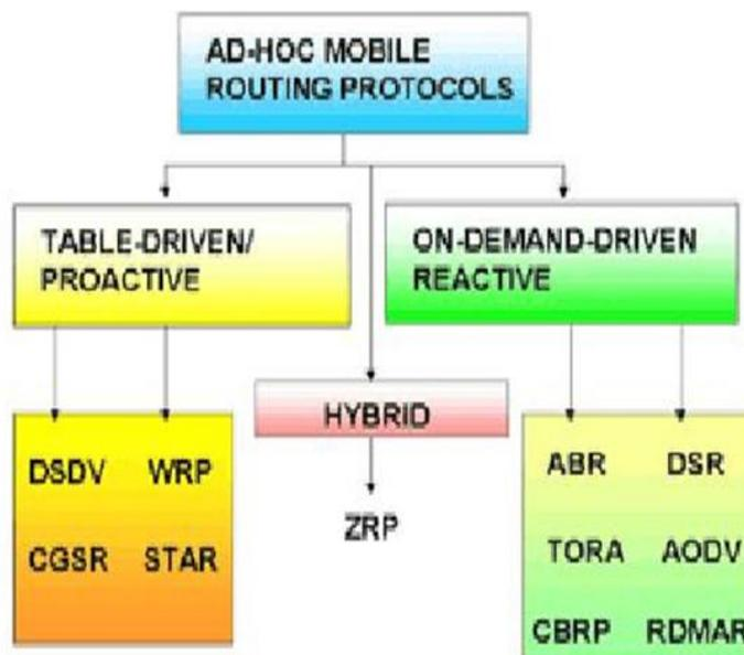
Fig 4-Ad-hoc Mobile Routing Protocols
